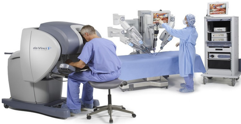
Figure 1. The Da Vinci robotic surgical system, which includes a surgical arm (right) and a separate surgeon console (left).
